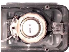
Mounting speaker in hood of engine using a metal grill for the exhaust.
