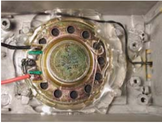
Mounting a speaker facing out from inside of the body. You have to seal all edges of the speaker for a proper baffle.
