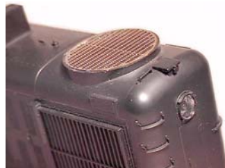
Mounting speaker in hood of engine using a metal grill for the exhaust.
