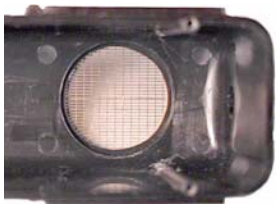
Mounting speaker in hood of engine using a metal grill for the exhaust.
