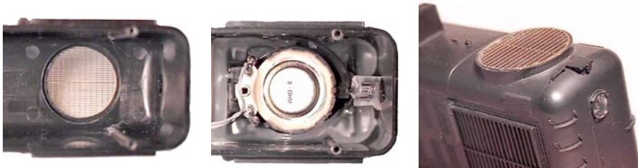
Mounting speaker in hood of engine using a metal grill for the exhaust.
