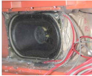
For open body shells it is necessary to make a speaker baffle instead of using the body for a baffle. In both cases, the backside of the speaker is closed off.
