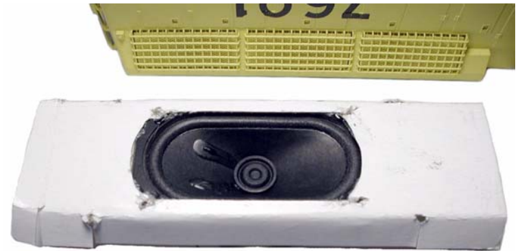
cardstock baffle - glue speaker gasket to baffle
