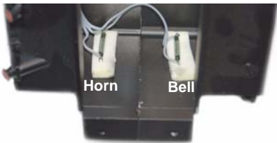
Bell Reed Switch in front of fuel tank.
