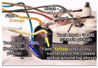
**Help for AF series motors.** Colors indicated are the #400 eunit connector and not the locomotives existing wires.
