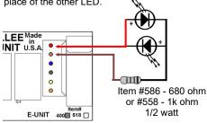
dwg #3 - directional LED's. If only one LED is desired you need to use a diode, #374, in place of the other LED.
