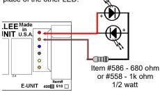
dwg #3 - directional LED's. If only one LED is desired you need to use a diode, #374, in place of the other LED.
