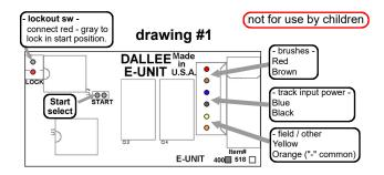
**Step#1:** Install the E-unit where as much free air space exists, using the attached mounting tape. For best adhesion, degrease the area first, then being very careful that no bare wires or other metallic objects come in contact with the components or the circuit board, mount the E-unit. If any contact is made to any metal object or stray wire while powered up, damage will occur to the E-unit. If you need to get better clearance, use more double sided tape (item 388).
