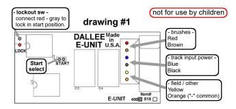
**Step#1:** Install the E-unit where as much free air space exists, using the attached mounting tape. For best adhesion, degrease the area first, then being very careful that no bare wires or other metallic objects come in contact with the components or the circuit board, mount the E-unit. If any contact is made to any metal object or stray wire while powered up, damage will occur to the E-unit. If you need to get better clearance, use more double sided tape (item 388).
