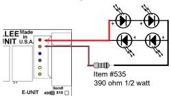
**dwg #3A** - 2 directional LED's. If only one direction pair of LED's is desired you need to use a diode in place of the other LED's.
