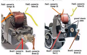
in later production type diesel or steam locomotives with a "hot chassis", make sure the ground/chassis plates (or anything else) do not contact the brush wires! This will damage the E-Unit.
