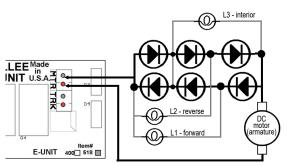
dwg #5 - 1.5 volt lamp directional headlights plus 1.5 volt constant lighting. The lamps MUST be insulated from the chassis. This configuration reduces the operating voltage to the motor.
