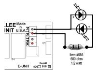
dwg #3 - directional LED's. If only one LED is desired you do need to use a diode for the other LED.
