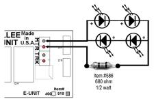
dwg #3A - two directional LED's. If only one direction pair of LED's is desired you do need to use a diode for the other LED's.
