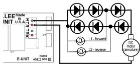
dwg #4 - 1.5 volt lamp directional headlights. The lamps MUST be insulated from the chassis. This configuration reduces the operating voltage to the motor.
