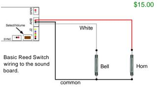
Connect Whistle/Horn and Bell reed switch wires to the three connector wires.
