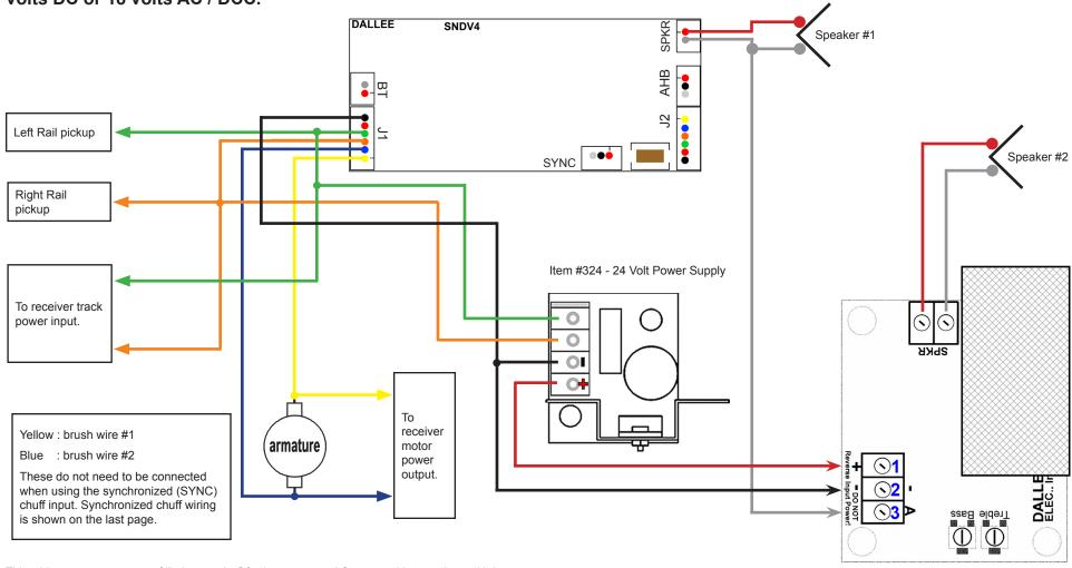
This wiring covers any type of "in locomotive" for larger gauge AC operated locomotives with item #672, 22 watt amplifier.
