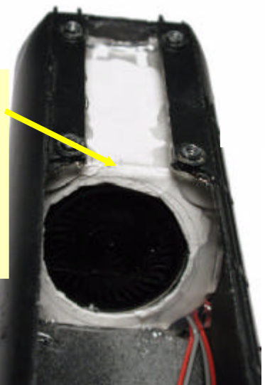
Speaker Baffle Use a piece of card stock to make a speaker enclosure. Seal all edges.
