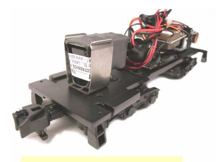
9vBRLT, installed upside down. Spread battery bracket slightly at it's base to allow for a snug fit. Don't spread too much or the tender shell will not clear.
