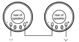
speaker connection speaker connection when mounting in a "B" unit or "dummy" place one speaker at each end - use the door as the opening.
