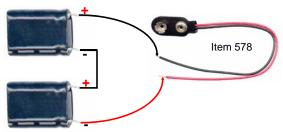
fig 1 - two Super Capacitors used to replace a 9 volt battery in MTH / QSI type older sound units. Before sequencing the engine, a 30 second wait is required to charge the super capacitor's. Tape the electrical connections or totally encase in heat shrink tubing to prevent shorts.
