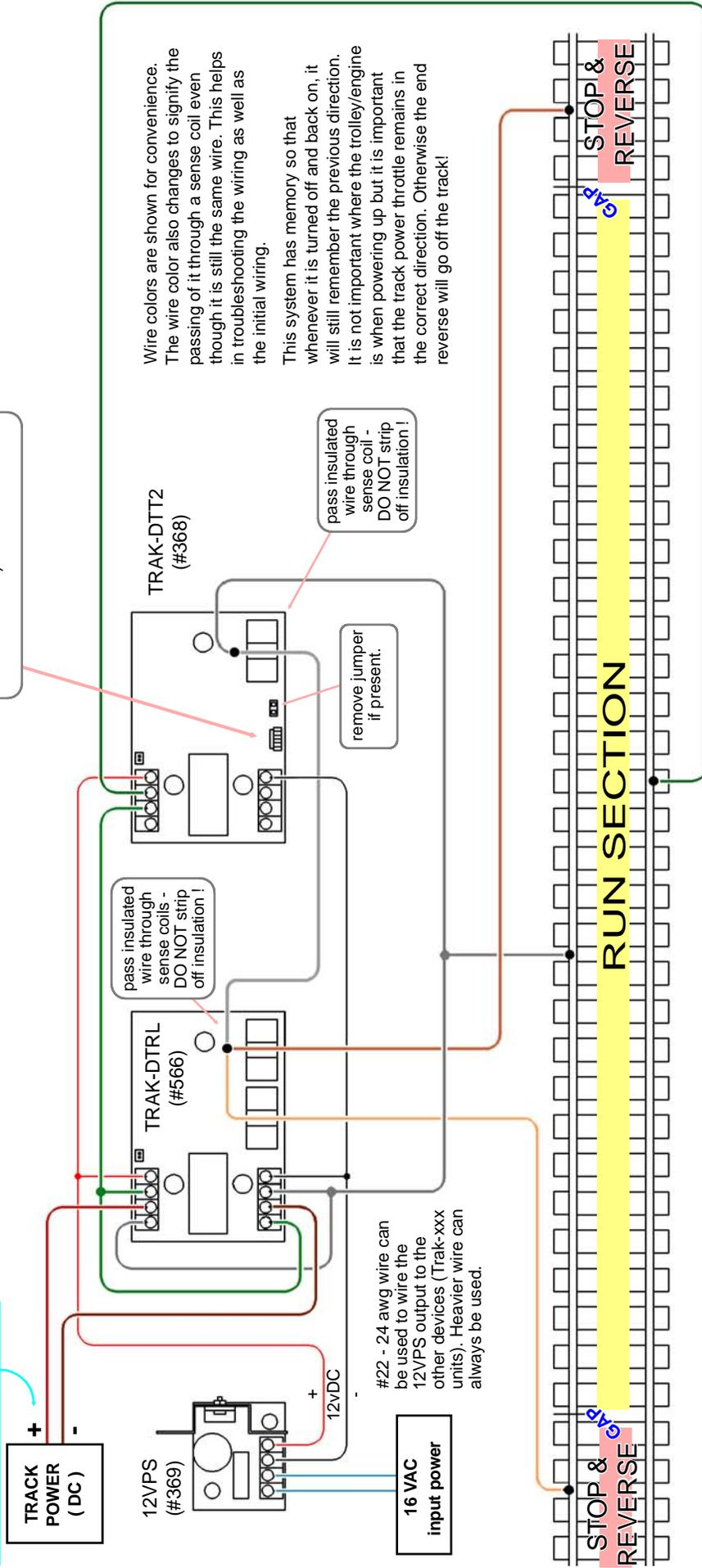
Wire colors are shown for convenience. The wire color also changes to signify the passing of it through a sense coil even though it is still the same wire. This helps in troubleshooting the wiring as well as the initial wiring.
