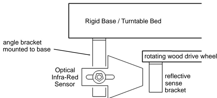
Exploded side view of bottom rotating wood drive wheel, showing optics aligned to stop bracket.
