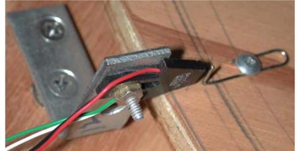
shown reading a paper clip or other rigid fine wire. Remember, the clockwise and counter clockwise stop resolution depends on the thickness of this metal (as discussed on page2).
