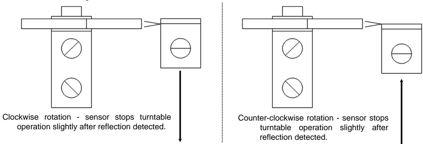
Sensor accuracy determined by thickness of sense bracket. If the bracket is located closer to center of the turntable bed, the error of stop position for clockwise versus counter-clockwise becomes greater. In some cases it may be necessary / desirable to overshoot the stop position and reverse the table for accuracy in one direction only.
