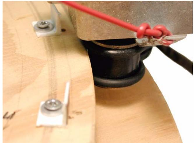
By applying drive O rings top and bottom of the drive wheel the turntable bottom maintains a proper elevation for the optics to read. A wandering disc prevents the optics from proper reading.
