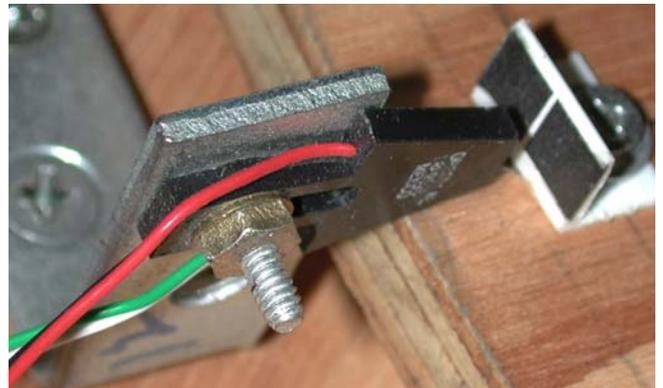
If you choose to use the laser printed laser stripes, the brackets would be mounted as shown above. In this picture plastruct plastic angle brackets used. First they were cut to size. Then large, or oval, mounting holes were drilled. Last, the laser printed stops were placed on the brackets face.
