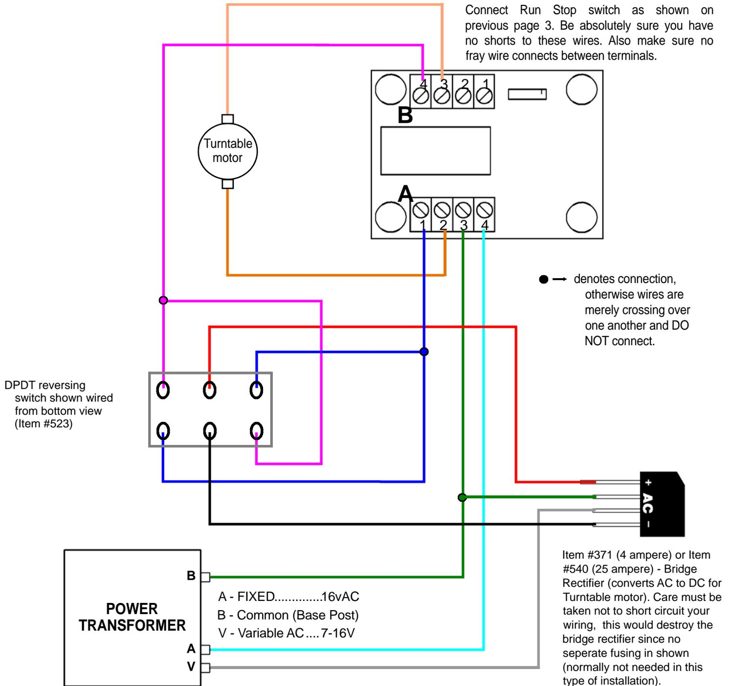
If a direction switch is not desired, wire the bridge rectifier "+" to barrier strip "B" #4 and the bridge rectifier "-" to barrier strip "A" #1. If the turntable rotates in the opposite direction desired merely reverse the wires on the motor.
