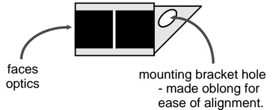
The optics do not sense black or the lack of focus, they do however sense any reflection of light striking the optical pickup. This light is generally the infra-red light generated by the internal infra-red led. It will however also sense ambient light striking the sensor, since that also contains infra-red light as well.. So care must be taken when alignment is done so that ambient light does not strike the sensor.
