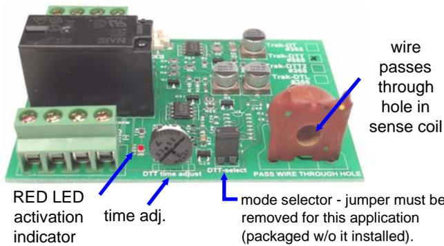
Install wires by stripping insulation back 3/16", place wire in hole, run screw down (CW) to clamp in position. Best to use stranded wire. Suggested wire sizes: Signal type wires can be 24 - 30 awg, 12vDC and other medium loads: 20 - 26 awg, Power type wires: 12 - 18 awg.
