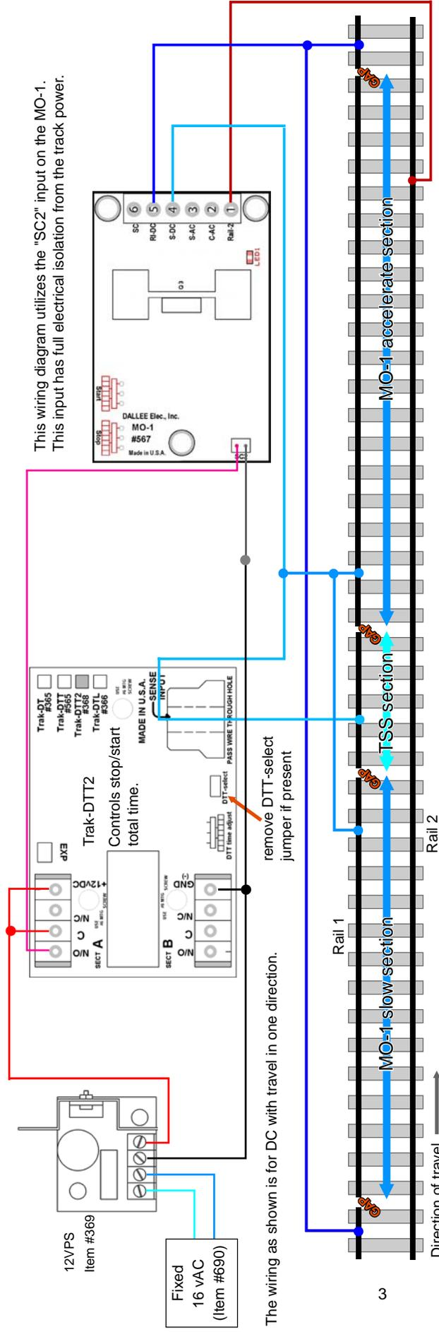
This wiring diagram utilizes the "SC2" input on the MO-1. This input has full electrical isolation from the track power.
