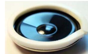
Body shell after speaker installation. Speakers are mounted on a card stock formed shelf and then hot melted in place. Air space is required between the front of the speakers and the body bottom but the back of the speaker enclosure is completely sealed to make a good enclosure! This type of installation yields more sound per watt than one single speaker.
