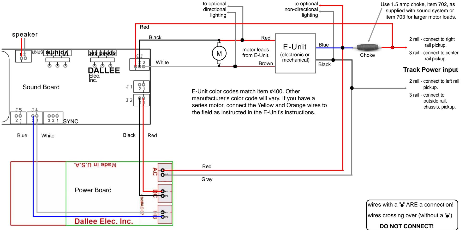
If you do not want the sound system to operate from the standard Horn/Bell signals, then disconnect the HB - J4 wire harness.
