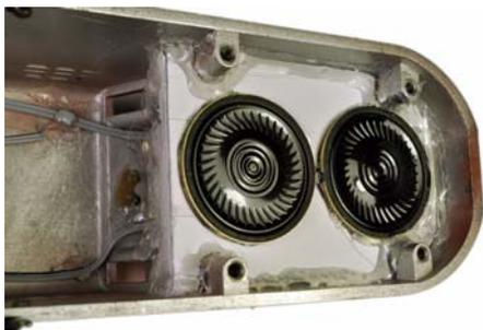
The two ends have their speakers wired in series. These two ends are then joined together back at the sound systems speaker wires. The top pair shown in the schematic below are the one sides speakers. The lower pair are the opposite end. The speakers utilized are item 661.
