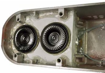
Top side of speakers with speakers and baffle totally sealed with glue. Note how the wires are held into place with dabs of glue. Their exit from the baffle is also totally sealed against any air ape.
