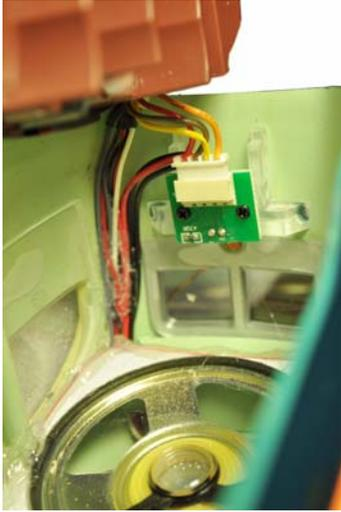
After gluing the speaker to the baffle piece, then locate it properly inside the shell. The wires are also tacked in place before to make sure they stay in place. For this we used hot melt. If you don't feel you can operate a hot glue gun very well, then use "Quick Grip" which is found in the craft shops. Quick Grip is nice since it never hardens fully and does set rather rapidly. We use it for a lot of projects.
