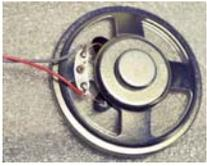
Before gluing the speaker to the template, properly solder wires to the back of the speaker as shown. These wires then need to be routed beneath the template's folded edge along the lighting strip to plug into the sound unit.
