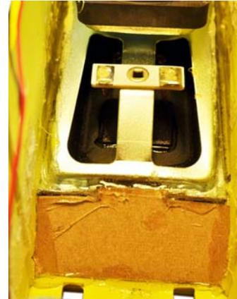
Step 6: Cut another piece of stock for the other end. This piece is about 2.2" x 1". Then glue it in place at an angle as shown in the picture to the left. Again, make sure that all of the glue areas are air tight.
