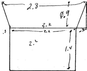
The first step is to make a rigid piece to enclose the hood end (of the engine) of the speaker. In this installation example, we used thick cardstock. This is to seal off any air leakage from the front of the speaker and shell. The template above is an exact size for doing this. You can either cut it out to glue it, or trace it, onto the piece you are using. It's important to use a thick piece since you do not want it to flex when the speaker is operating.
