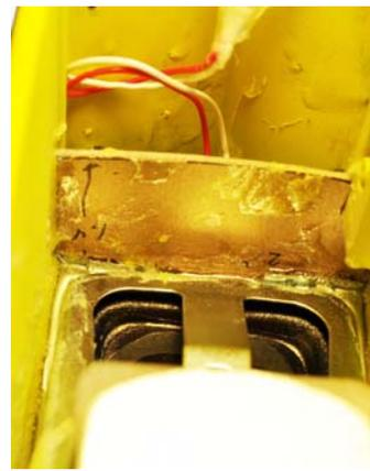
Step 4: Carefully cut the metal tabs off of each end of the speaker (item 217) leaving the ends flush and straight. Then place the speaker into the shell placed tightly against the first baffle piece. It is the perfect width for this shell as well.
