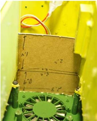
Third, install the fan assembly making sure it is securely screwed fastened and air tight. If you like, you could put some rubber based glue along the edge when assembling. Remember, you won't be able to get to the screws after the speaker is installed. This is shown in the picture on the left.
