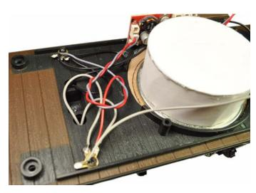
Position and glue speaker sides flush to the front with no air gaps as pictured.
