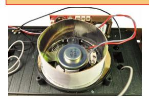
Position and glue speaker sides flush to the front with no air gaps as pictured.
