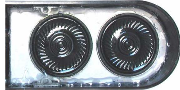
Body shell after speaker installation. Speakers are mounted on a card stock formed shelf and then hot melted in place. Air space is required between the front of the speakers and the body bottom but the back of the speaker enclosure is completely sealed to make a good enclosure / baffle! This type of installation yields more sound per watt than one single speaker.
