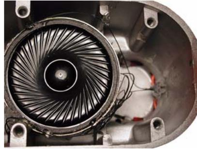
For open body shells it is necessary to make a speaker baffle instead of using the body for a baffle. In both cases, the backside of the speaker is closed off.
