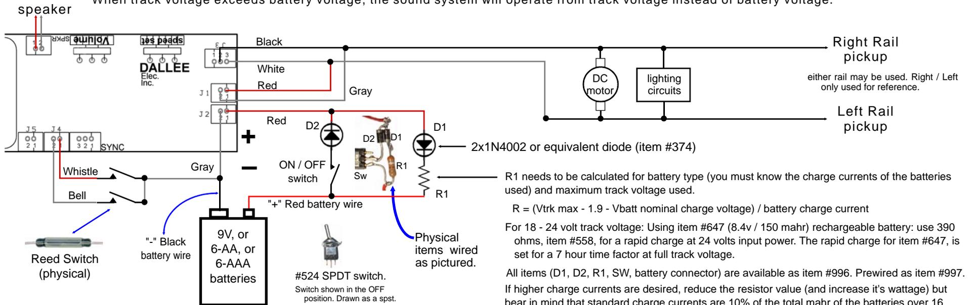
Battery power - must not exceed 35 volts DC. Use one 9 volt battery or a string of 6 AA or AAA batteries. Battery life depends on the volume setting and speaker impedance. Typical operation of most sound systems, with one good 9 volt battery, is about 8 hours, AA or larger mahr (milliamper hour) batteries is well beyond 50 hours!
