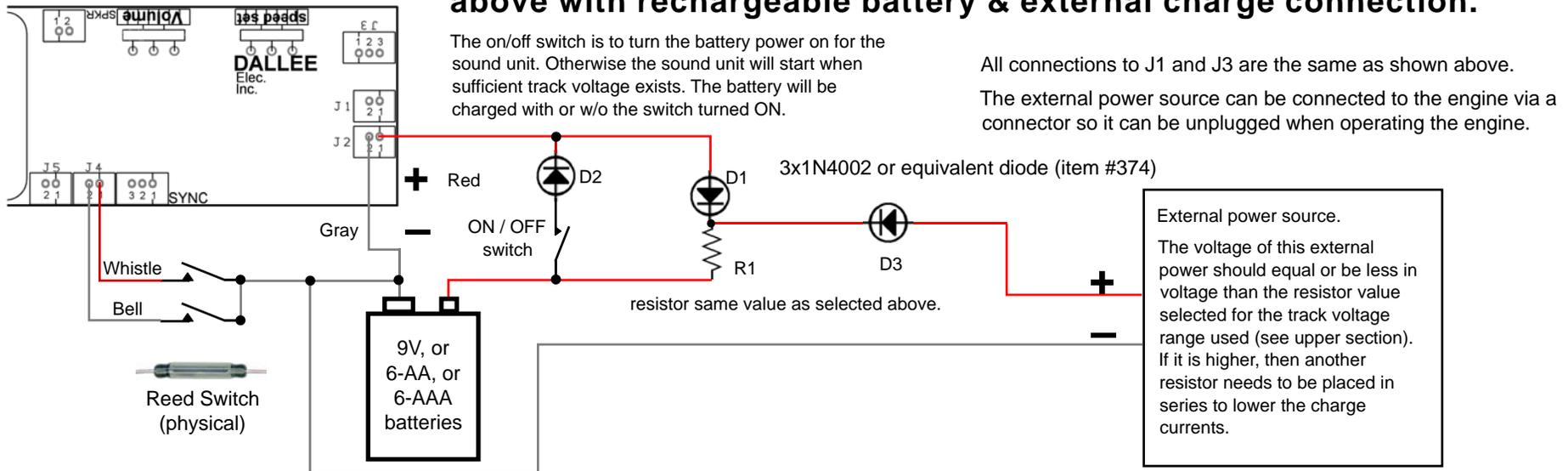
The on/off switch is to turn the battery power on for the sound unit. Otherwise the sound unit will start when sufficient track voltage exists. The battery will be charged with or w/o the switch turned ON.
