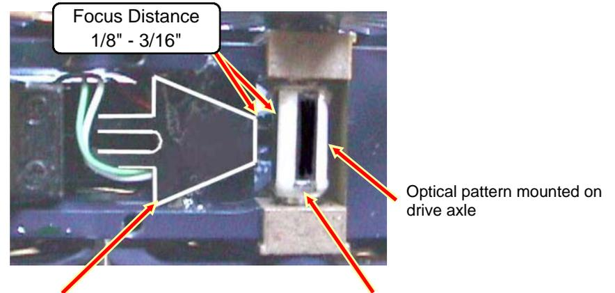
Optical Coupler, item 583 (hi-lighted for ease of viewing), mounted to frame 3/16" from optical end to pattern. In this installation, the end mounting ears had to be trimmed to obtain clearance to the drive gear box. When doing so care must be used to not damage the optics.
