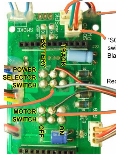
"SPKR" : Speaker connector. Connect to Sound units "SPKR" connector wires.
