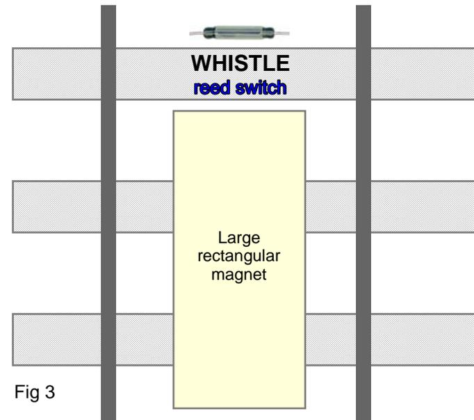
Since magnet strength and reed switch sensitivity varies, you may need to adjust placement to suit your needs. The basic scheme is shown for proper magnet placement. Do not place magnets exactly opposite of each other.
