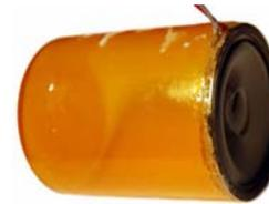
**Speaker enclosure:** Normally the shell of a tender sealed to the base will form an enclosure. However, if this is not ideal, a pill bottle with it's end cut, as shown, off makes a nice enclosure as well. Be sure to seal the entire edge around the speaker to the bottle. The wires come through a small notch placed in the lip so that they do not become pinched from the speaker.
