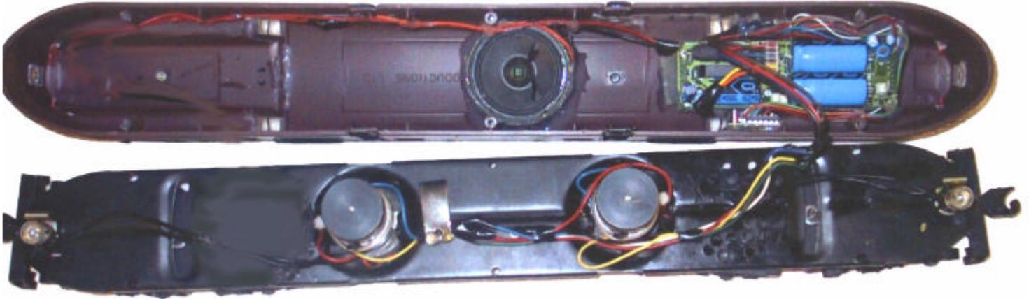
As can be seen, plenty of space is available inside a full scale GG-1. This unit shows the standard lamps that existed. A better option is to install the lamps that were supplied with the LocoMatic™ system.
