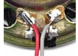
when soldering wires to rear of speaker, care must be taken so that the wires do not come in contact with the speakers metal frame!
