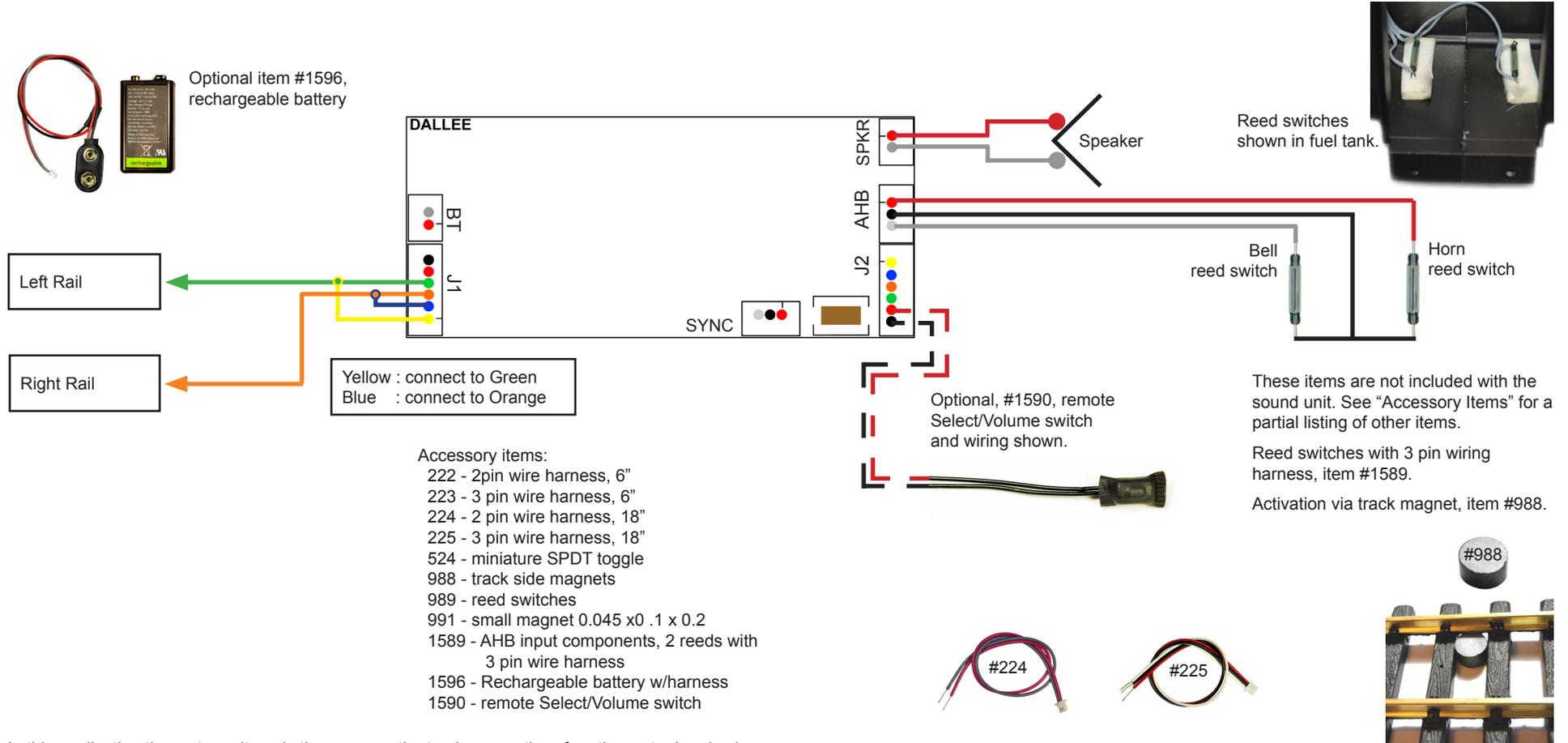
In this application the motor voltage is the same as the track power, therefore the motor brush wires (Yellow and Blue) are wired to the track power wires (Green and Orange) as shown.
