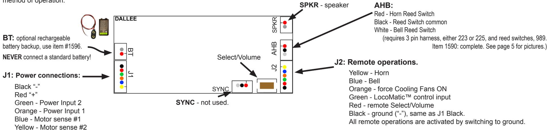
The following connectors all connect to the J1 Black wire, which is the sound units ground ("-") reference. These are connected internally on the board and do not need to be connected externally!
