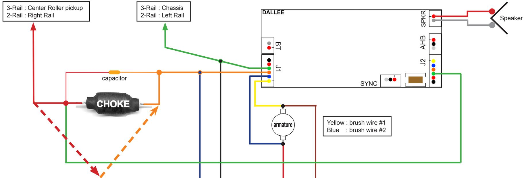
Wiring for AC track power is exactly the same as previously done with the exception of the choke and capacitor being added in series with the track power. The large RED dashed wire represents connections to all other present loads inside the engine. This would be lights, smoke unit, etc.. They must be disconnected from the track pickup power and reconnected to the orange wire above, after the choke. This change in wiring is shown as a dashed line.
