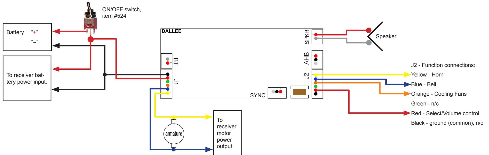
This wiring covers any type of radio receiver operating on the same battery power as the sound unit. Since both are operating on the same power, and both units share the same ground (common). This is why the black wire from J2 does not need to connect to the receiver.
