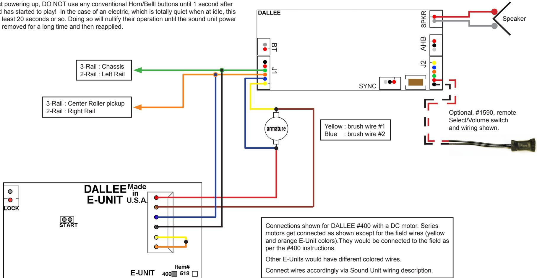
Wiring for AC track power is as simple as shown. The brush wires remain connected to the existing E-Unit and also to the sound unit as shown. Which brush wire is used for #1 or #2 is not of importance. Failure to connect these wires will result in the sound unit's Cooling Fans to remain off regardless of the motor / engine speed.
