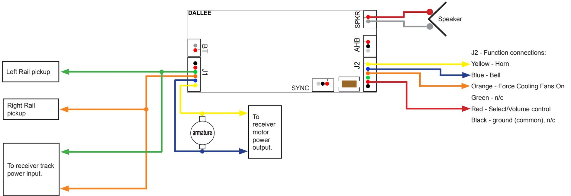
This wiring covers any type of radio receiver or DCC decoder operating on the same track power as the sound unit. Since both are operating on the same power, and both units contain a bridge rectifier (normally they do), then both share the same ground (common). This is why the black wires from J1 and J2 do not need to connect to the receiver ground. Doing so will not cause any problems.
