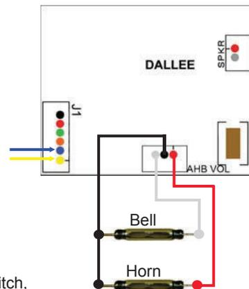
For Auto-Horn / Bell track magnet operation, use item #1589 with item #988 track side magnets.
