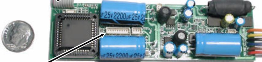
**Lighting outputs for headlights, markers, cab, interior, etc..** All lighting is set for a 5 volt constant output. Seven controlled via the microcontroller, or as an option\* six can be controlled by you the user! Two miniature 5 volt lamps included. LED's with resistors may be used. **Contains all motor power and control with sound on one main board with remote board for Volume and option selection.**
