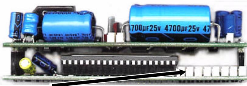
**Lighting outputs for headlights, markers, cab, interior, etc..** With one constant 5 volt output, seven controlled via the microcontroller, or as an option\* six can be controlled by you the user! All lighting is set for a 5 volt constant output. Two miniature 5 volt lamps included. LED's with resistors may be used.
