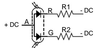
Method 2: using 2 resistor's in series with each cathode. Required to balance the led's when both are illuminated.
