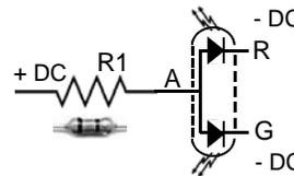
Method 1: using 1 resistor in series with the common Anode.
