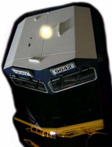
Our new STROBE features an Incandescent White T1 3/4 (5mm) LED with a super bright output of over 12,000 millicandella lamp power! This is great for the outdoor model railroader as well as indoor. Incandescent White means that it has the color of a standard lamp and not the blueish color associated with other so called "white" LED's.
