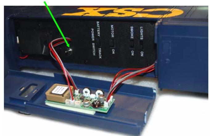
6 - as can be seen above, the sound board is easily mounted in the switch access roof panel. It not only clears all of the other switches when mounting this way, but access to the volume and notch setting controls are easily accomplished. As can be seen, all wires to the sound board pass through the existing openings.
