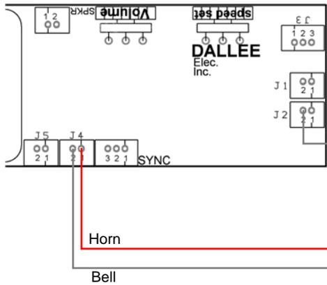
Basic Reed Switch wiring to the sound board.
