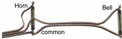
2 - Since one reed switch controls the Horn and the other controls the Bell, they need to be mounted on opposite sides of the chassis. These are shown below, attached with double sided tape (item 388), inside the fuel tanks end. To keep things consistent, we used the right side of the engine for Horn activation and the left for Bell. By wiring all engines the same way, it is easy to know which side activates which function.
