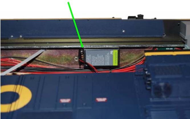
5 -A sound on/off switch (item 524) can be easily mounted by drilling a small hole in the shell as shown. Place it in the same direction as the other switches. This way the "ON" position will be easily known.
