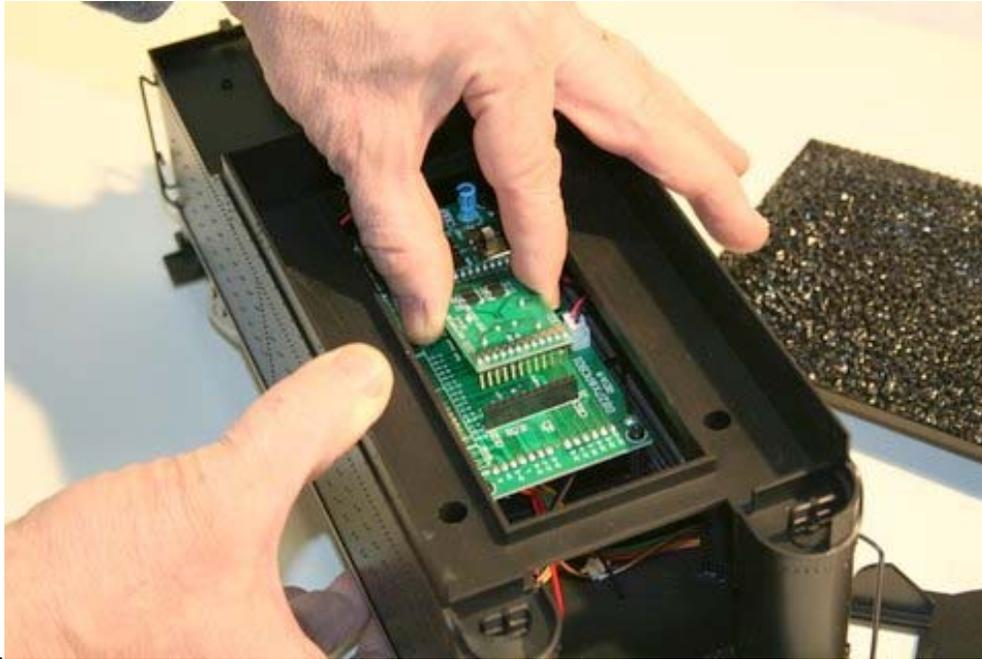
To install the Dallee Steam Sound decoder, connect the Dallee AC input J1 leads to the J1:1-12 solder pads on the (DC) Dummy PC Board. The gray wire goes to **J1:1** and the red wire to **J1:12**.
