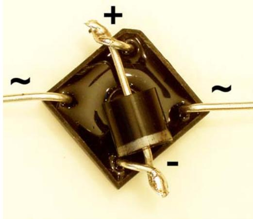
Install the rectifier in one motor lead in the K27. The easiest way to do this is to cut the **orange motor M+ wire** and connect one end of the wire to each ~ lead as shown in the photo below. The photo also shows the Dallee Steam sound board installed using the dummy socket reinstalled in the socket on the main PC board in the tender.
