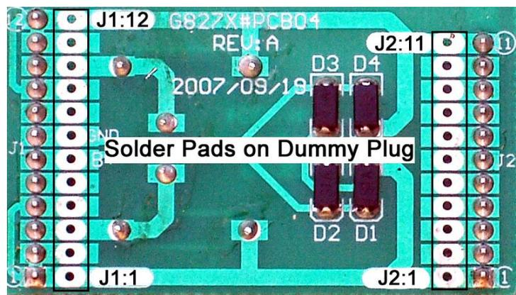
If you wish to use the Dallee automatic chuff synchronization connect the Black and White wires of the J3 connector to the J1:2-11 pins the black wire going to **J1:2** and the white wire to **J1:11**. If you wish to use the locomotives optical sensors you do not need to make these connections.
