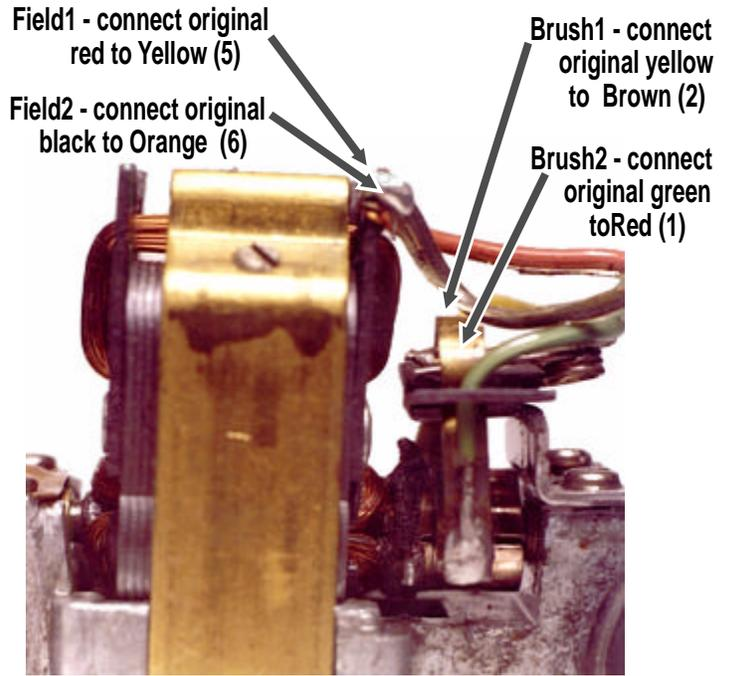
**Help for Lionel series motors.** These pictures show where the grounded field wire needs to be broken from the chassis for the motor power. Left picture is early Lionel. Right is later series motor style. It is always better to add a ground wire to both outside rail pickups and the chassis. When more than one center roller is available always connect to both, also secure the center pin from rotating with the roller.
