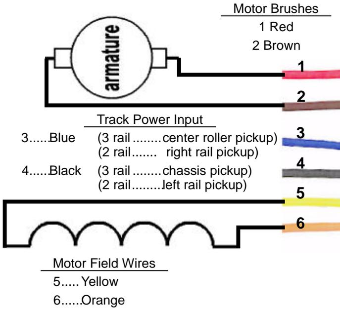
If the engine does not have a chassis (outside rail) pickup from each truck you should add one to prevent intermittent track pickup from occurring. Adding multiple center rail pickups will also help.
