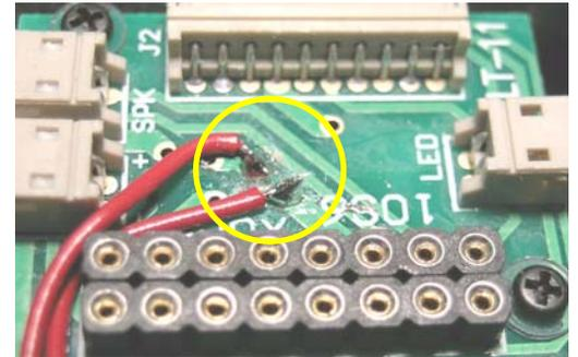
Step 3: Tin the copper tracks and attach wires from motor reduction circuit as built below. Be careful not to create a short to an adjacent track.
