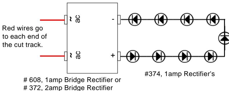
The number of diodes, #374, determines the speed reduction. A good low speed requires 9 diodes placed in series as shown. Fewer diodes will allow for a faster running engine. The parts must be soldered into a small package as pictured below.
