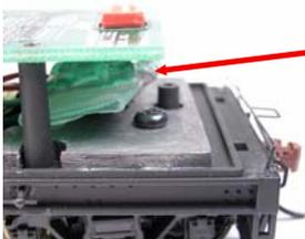
When finished, and wires are attached to the pcb, tuck the diode drop assembly on top of the rear weight as shown. This does get quite warm when operating the engine.
