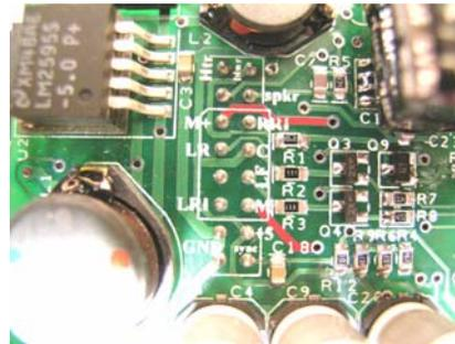
Step 2: Locate the motor power tracks, highlighted in RED. The end of each motor track is labeled as M+ and M. Cut only 1 track (whichever you feel is easier to utilize). Scrape the green insulation to reveal bare copper. Attach the wires from the motor reduction circuit similar to Step 3 above.
