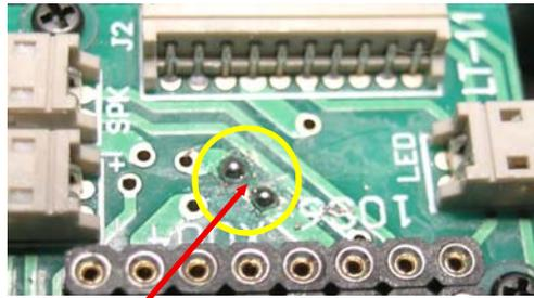
Step 2: Cut Track. Scrape the green insulation to reveal bare copper and tin as shown.
