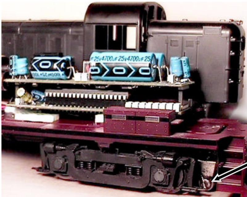
For best operation, secure center roller pickup to the roller's pin. Do this on both pickups. File the side of the pin to allow the Rosin core solder to quickly clean and allow the solder to flow without melting the plastic support.
