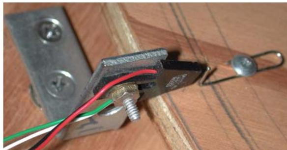
Shown reading a paper clip or other rigid fine wire. Remember, the clockwise and counter clockwise stop resolution depends on the thickness of this metal.
