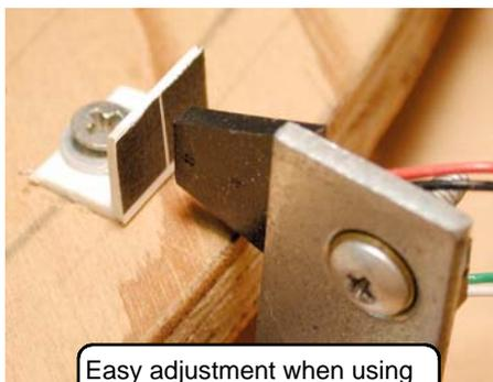
Easy adjustment when using a large flat head screw or a screw with a flat washer.
