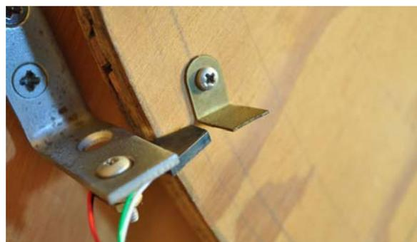
Shown reading an angle bracket. Remember, the clockwise and counter clockwise stop resolution depends on the thickness of this metal.
